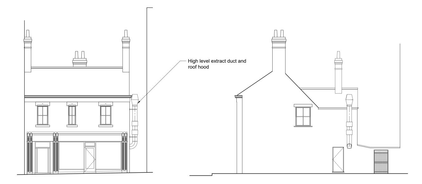
Proposed Main (South) Elevation Proposed Side (East) Elevation
